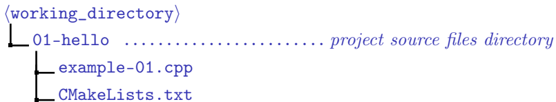
Figure 1: structure for the simple project directory
