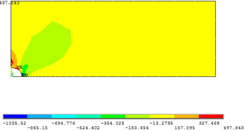
Figure 5. Distribution of axial stresses  $T_{yy}$
