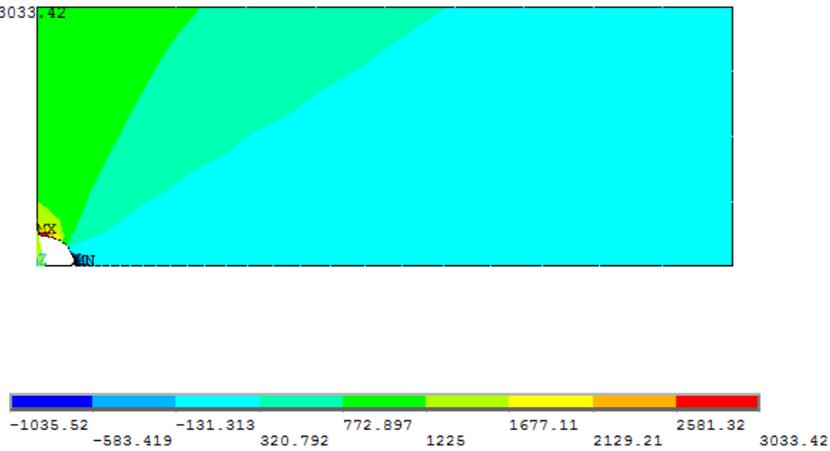
Figure 6. Distribution of tangential stresses  $T_{\theta\theta}$
