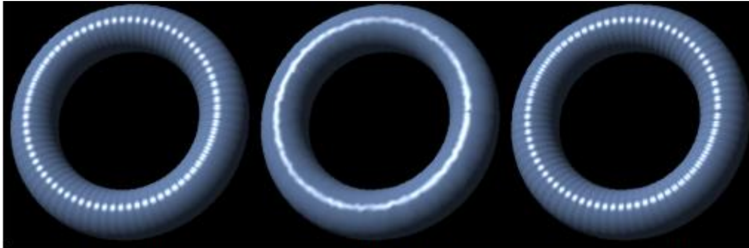
Figure 1: Bumpy Torus Model. Left : 44,252 triangles full resolution mesh. Middle and Right : 5,531 triangles, 0.25 mm maximum image deviation. Middle : per-vertex normals. Right : normal maps
