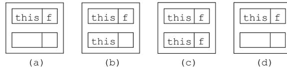
Figure 3.3.: Successive frame states for the `setF` method: a) initial state, b) after `ALOAD 0`, c) after `ILOAD 1` and d) after `PUTFIELD`
