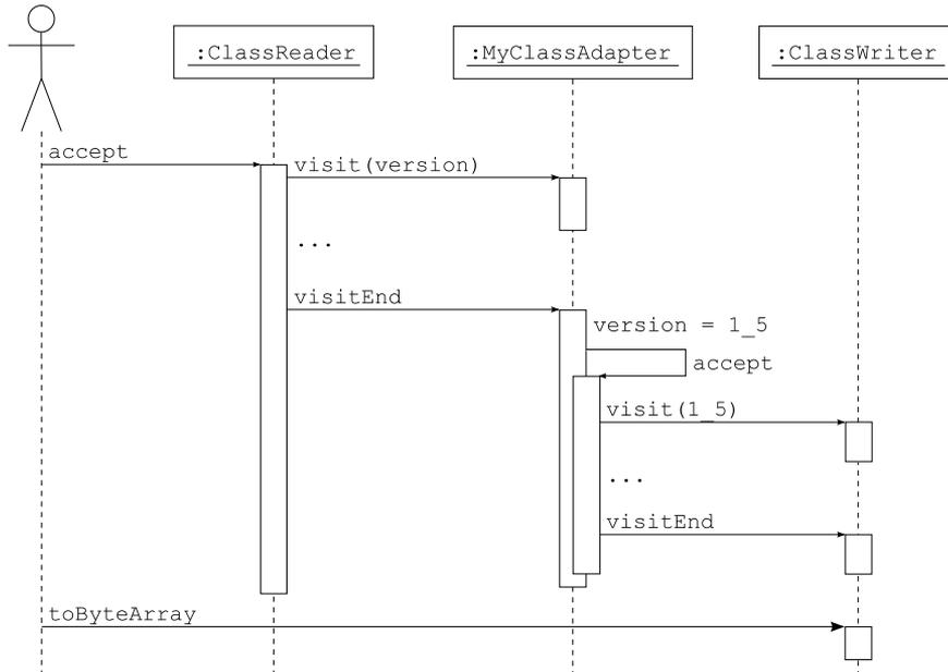
Figure 6.2.: Sequence diagram for `MyClassAdapter`
