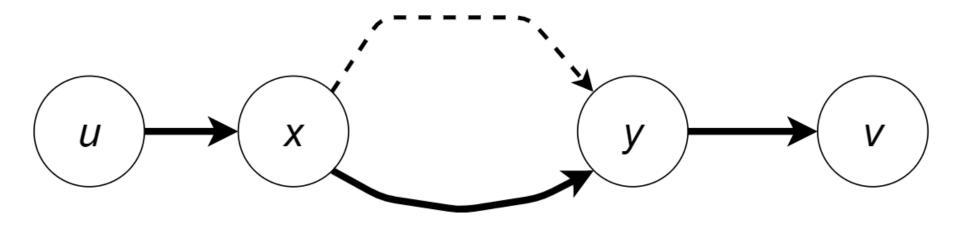
Due to the principle of optimality, the shortest paths from a given source vertex to all other vertices make the *shortest path tree*.
