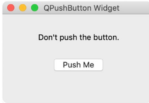
Figure 3-3. Example of the QPushButton widget
