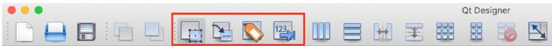
Figure 7-10. Qt Designer’s Editing Modes (outlined in red). (From left to right) Edit Widgets, Edit Signals/Slots, Edit Buddies, Edit Tab Order
