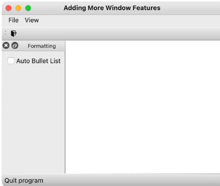
Figure 5-12. GUI with a toolbar, a status bar, and a dock widget. The status bar on the bottom displays the text “Quit program” when the mouse hovers over the Quit icon in the toolbar
