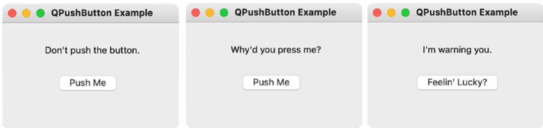
Figure 3-1. Clicking on the QPushButton will change the label's text and, eventually, the button's text
