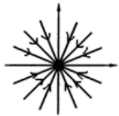
Special case: Stable Degenerate Star Node \lambda_1 = \lambda_2 is real and negative (many eigenvectors)
