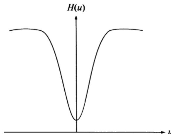
$$h(x) = \sqrt{2\pi}\sigma Ae^{-2\pi^2\sigma^2x^2} - \sqrt{2\pi}\sigma_2 Be^{-2\pi^2\sigma_2^2x^2}$$
