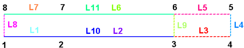
Figure 3.7. Line concatenation for a solid model of the meridional section of the disk
